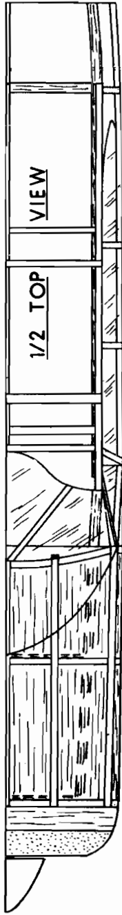
CENTER SECTION CONSTRUCTED ATOP FUSELAGE
