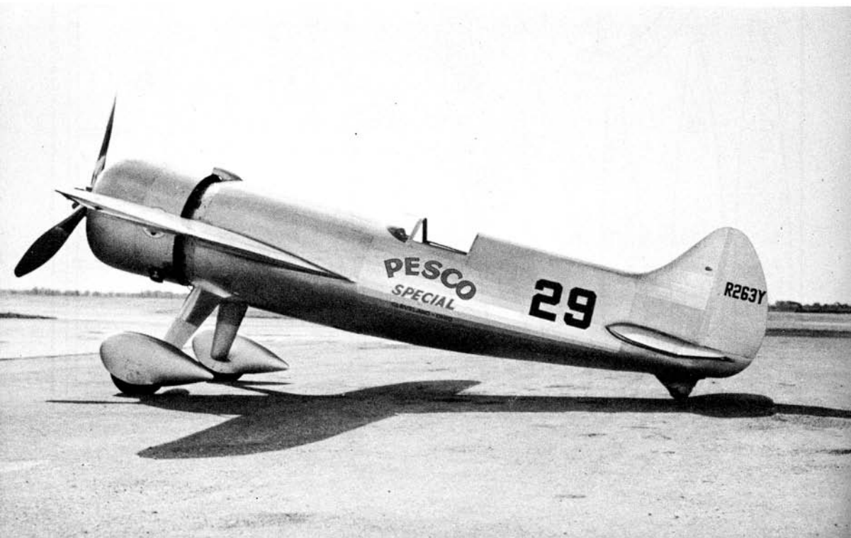
Two views of Colonel Roscoe Turner's famous Turner-Laird Pesco Special racer. Powered with a Pratt & Whitney Twin Row Wasp engine of 1,250 h.p., this ship has been a consistent winner in air races. The upper picture shows details of the landing gear and cowling, and in the lower the cockpit arrangement and fuselage shape may be seen. (William F. Yeager photos)
