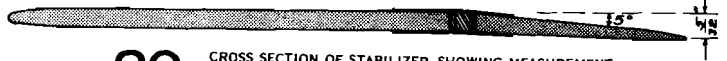
20 CROSS SECTION OF STABILIZER. SHOWING MEASUREMENT FOR MAXIMUM DOWN ANGLE OF ELEVATORS
