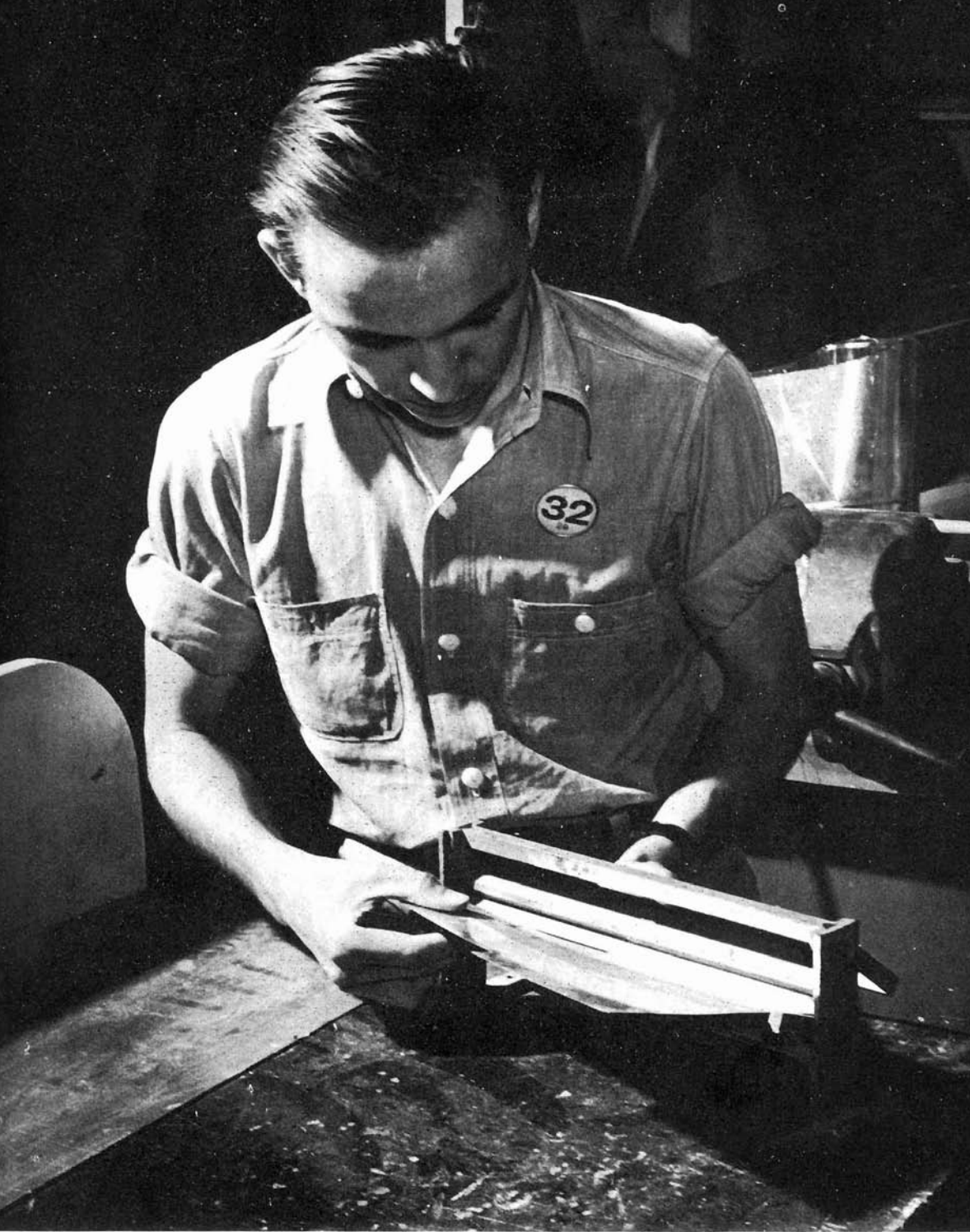
Harvey illustrates how one of the tools he and his brother made enables them to make a straight cut on a large sheet of metal. The models that are turned out by the twins are used by the Army and Navy for instructing flying cadets; Consolidated Vultee representatives throughout the world also use them.
