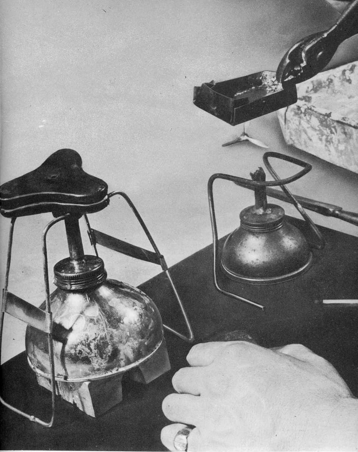
Furnaces improvised from oil cans and baling wire are used when molding the tiny propellers. The burner at the right is used to melt the metal, which is held above it in a special tray. Above the burner at the left is the mold into which the molten metal will be poured.
