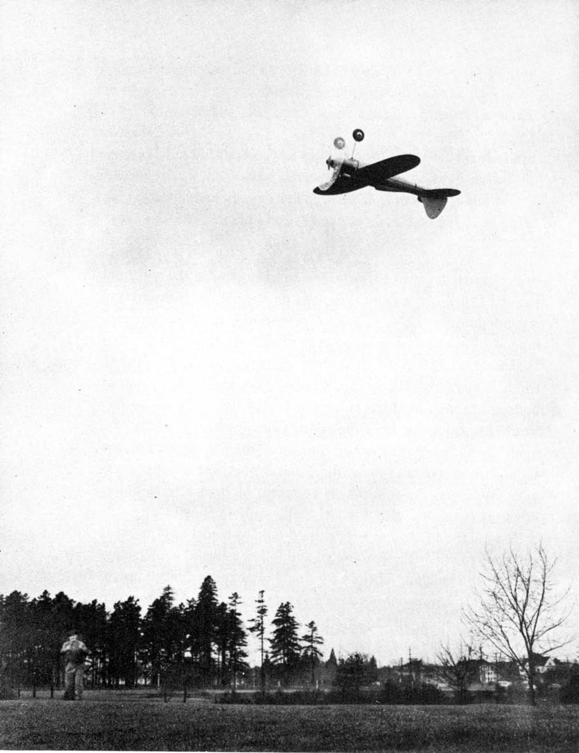
Jim Walker, designer and builder of the Fireball, flying his amazing little model upside down. With U-control, the Fireball can be put through a series of maneuvers which are impossible with the average model. Either a Class B or C engine may be used.
