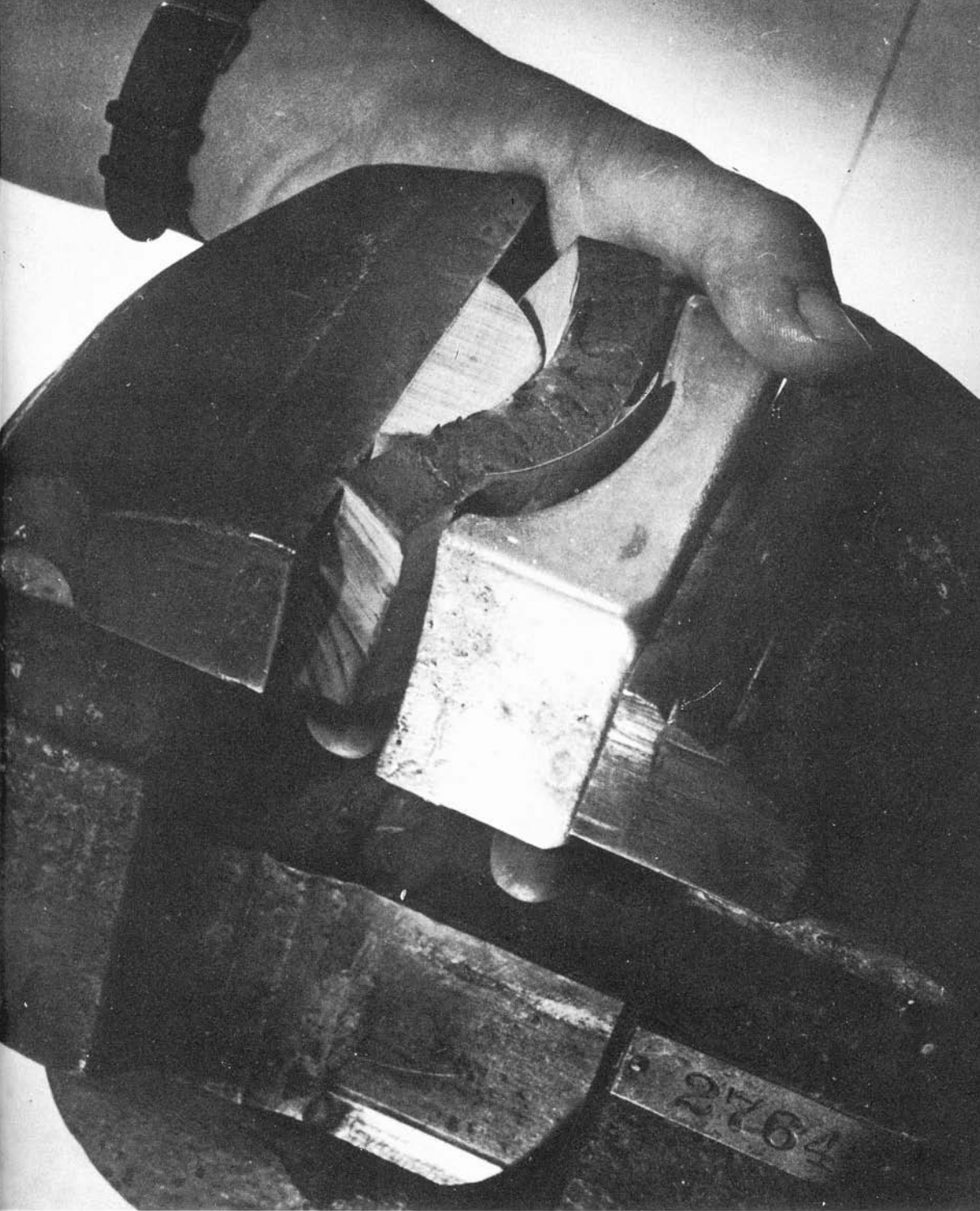
Bench vises provide the pressure for forming many of the assembly units. Here sheet sponge rubber, like that used on giant hydro-presses for full-size airplane parts, aids in the forming operation. Note also that a curved wood block is used behind the rubber.
