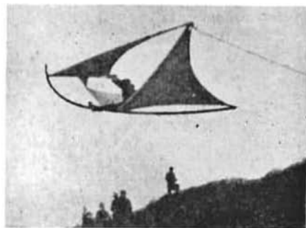
Fig. IV.—The sailplane stability and controls flight tested in captive flight in slope lift
