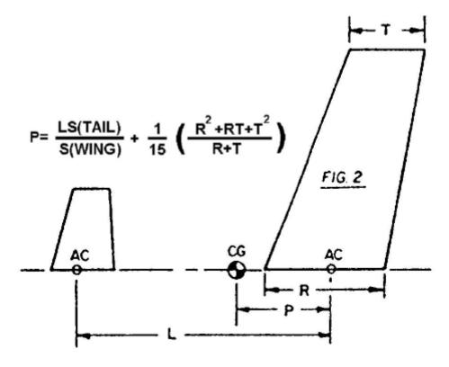
This center of mass location guarantees that the aircraft will basically stable in pitch. After test flights have been made, it may be desirable to move the center of mass toward the rear of the airplane in order to improve the pitch response of the aircraft.
