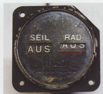
This device from Farnet, Grenchen, indicates the release status of the dolly and the towrope. Photo Thomas Fessler
